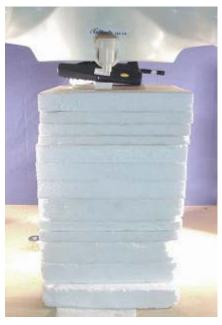
SAR Test Setup Back Side of EUT
