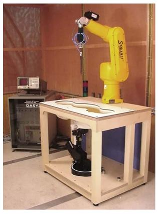
DASY3 SAR Measurement System with SAM phantom
