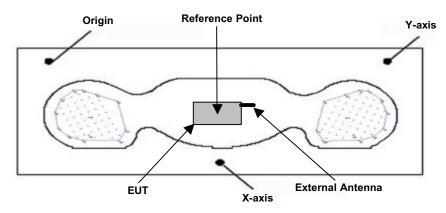
Figure 2. Phantom Reference Point & EUT Positioning - Back Side of EUT
