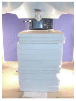
SAR Test Setup Right Side of EUT
