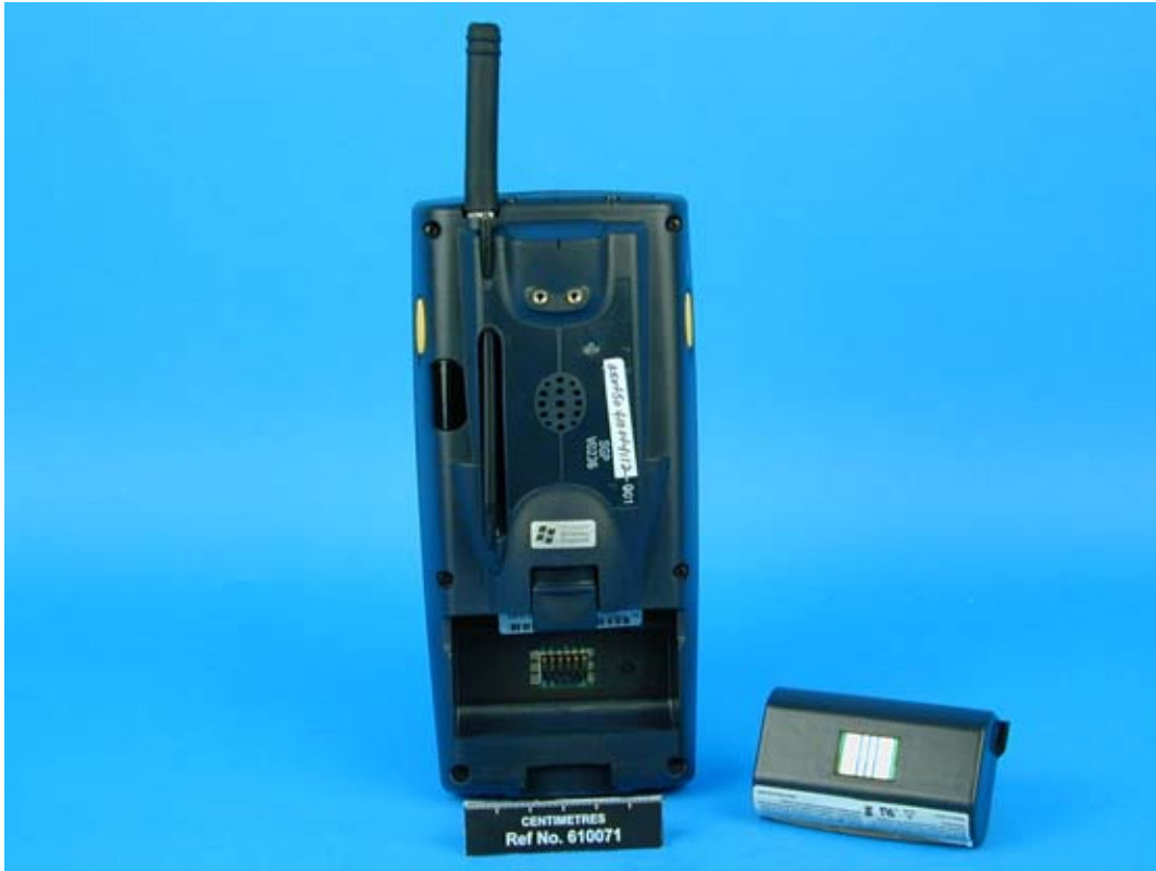
Figure 55. Rear View of the Intermec Handheld Computer Terminal, 700C-SMC45, with the battery removed.
