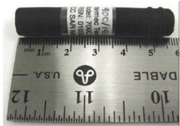
Dual-Band Stubby Antenna (P/N: 805-606-002)
