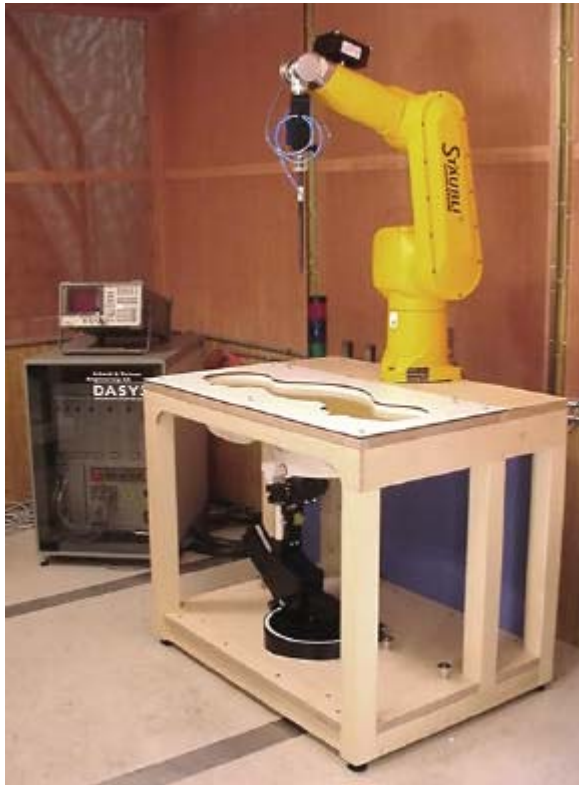
DASY3 SAR Measurement System with SAM phantom
