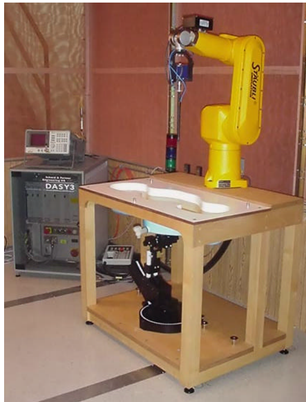
Fig. 5. DASY3 SAR Measurement System
