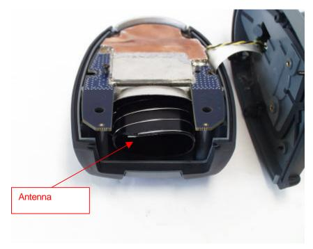
2. The handle was removed in the original SAR testing exactly like was done for the 1555-900 unit, which you approved 1/26/2001 refer to the SAR report for FCC ID HN21555-900. This was done to yield the maximum radiation exposure for "touching the surface of the antenna". There are no electronics in the handle which would effect the SAR data.
