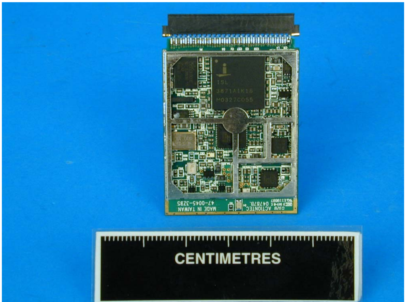
Bottom view of 802.11b Radio Module With Internal Cover Removed
