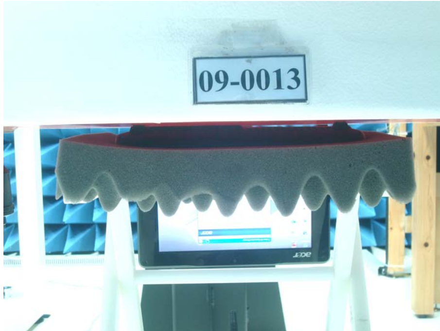
Figure 21. Body SAR Test Setup (Flat Section) _ EUT Bottom to Phantom 2mm space ( 3G Antenna to phantom 81.54mm space )
