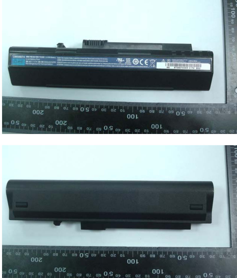
Figure 2. Li-ion Battery_UM08B74 5200mAh
