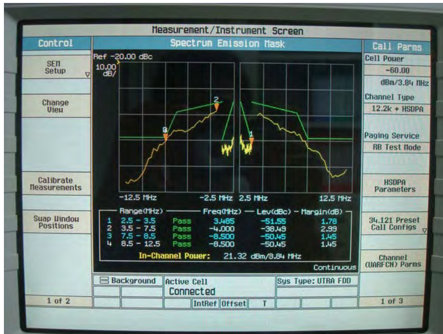
Figure 18. Spectrum Analyzer Flat HSDPA Band II CH9262
