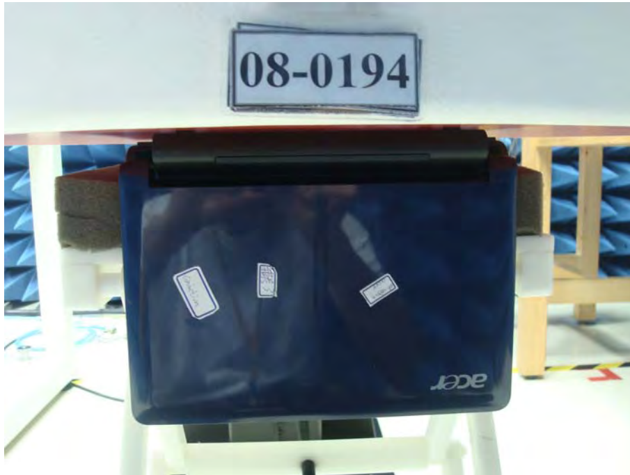
Figure 19. Body SAR Test Setup (Flat Section) _ EUT Bottom to Phantom 2mm space ( 3G Antenna to phantom 81.54mm space )
