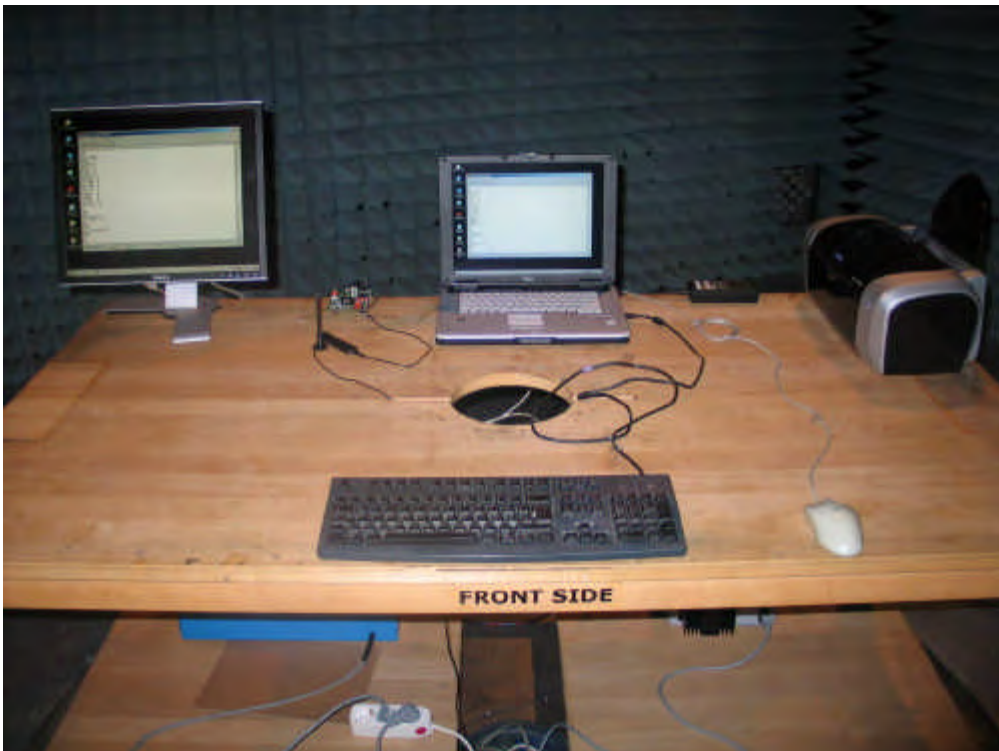
Photo 2: Test setup for radiated measurements
