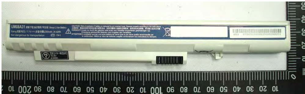
Figure 2. Battery (Li-Ion 11.1V , 2200mAh)
