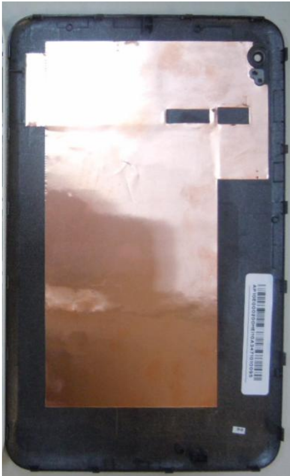
Fig.3 Original antenna window
