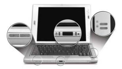
The battery, media and wireless communication status indicators are visible even when the LCD display is closed.
