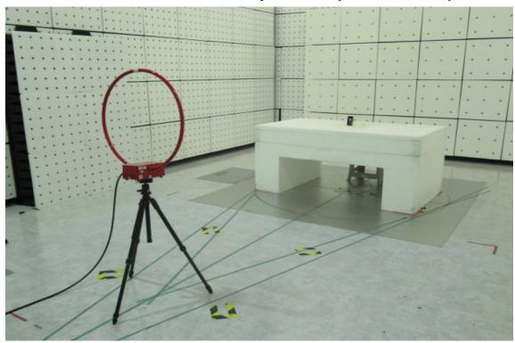
Radiated Emission Set up Photos (Below 1GHz)
