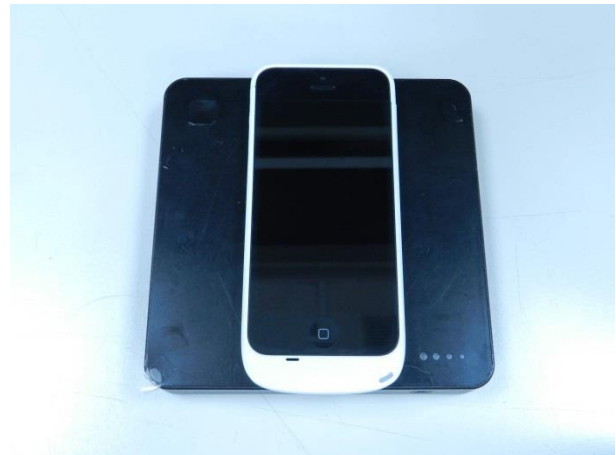
The Iphone5 with WPC back cover is placed on the EUT during the test.
