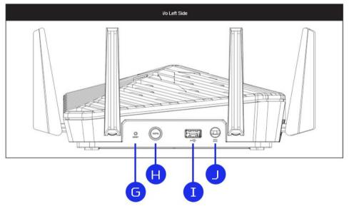
G: Pin Hole Reset Button H: WPS Button I: USB 3.0 Port J: AC Adaptor Port
