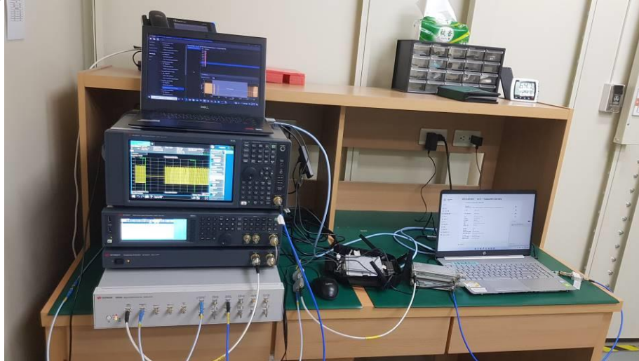
Photograph 9: Test Setup for CBP
