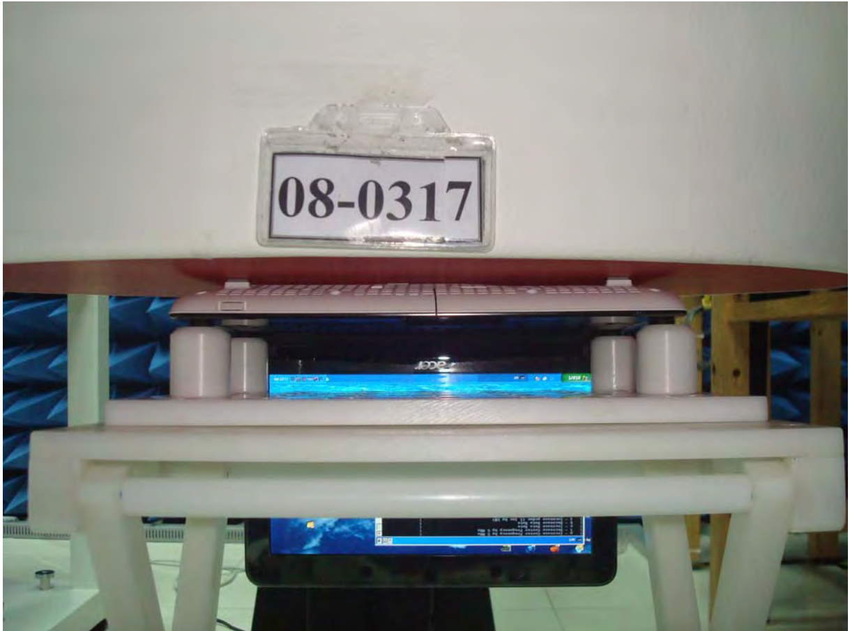
Figure 13. Body SAR Test Setup (Flat Section)
