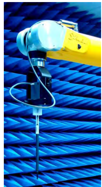
Figure 7. Probe setup on robot
