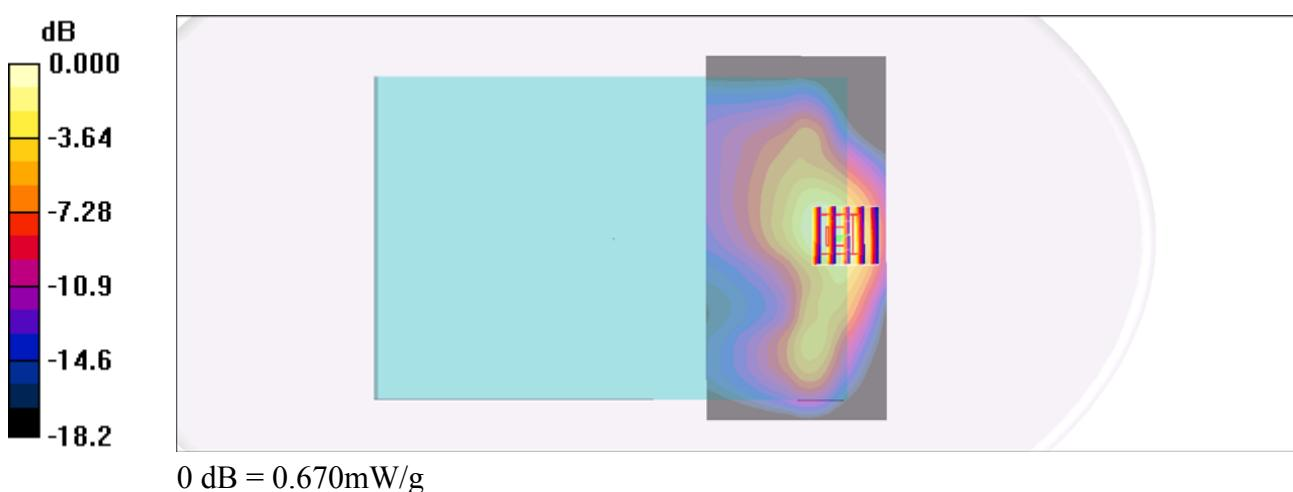
**#15 GSM1900\_GPRS10\_Bottom Face\_0.5cm\_Ch661\_Earphone****DUT: 132604-07**
