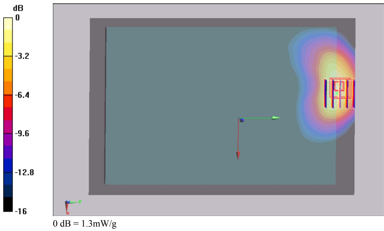
**#06 GSM850\_GPRS10\_Bottom Face\_0cm\_Ch251\_Earphone\_Down3dbm\_2D****DUT: 132604-07**
