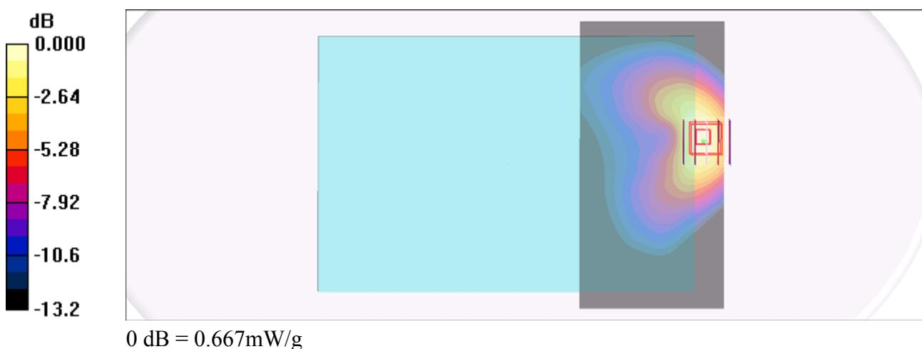
**#06 GSM850\_GPRS10\_Bottom Face\_0cm\_Ch251\_Earphone\_Down3dbm****DUT: 132604-07**
