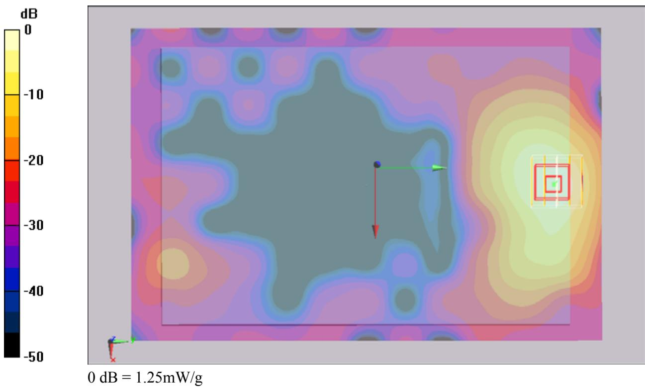
**#02 GSM1900\_GPRS10\_Bottom Face\_0cm\_Ch810\_Earphone\_Down4dbm\_2D****DUT: 132604-07**
