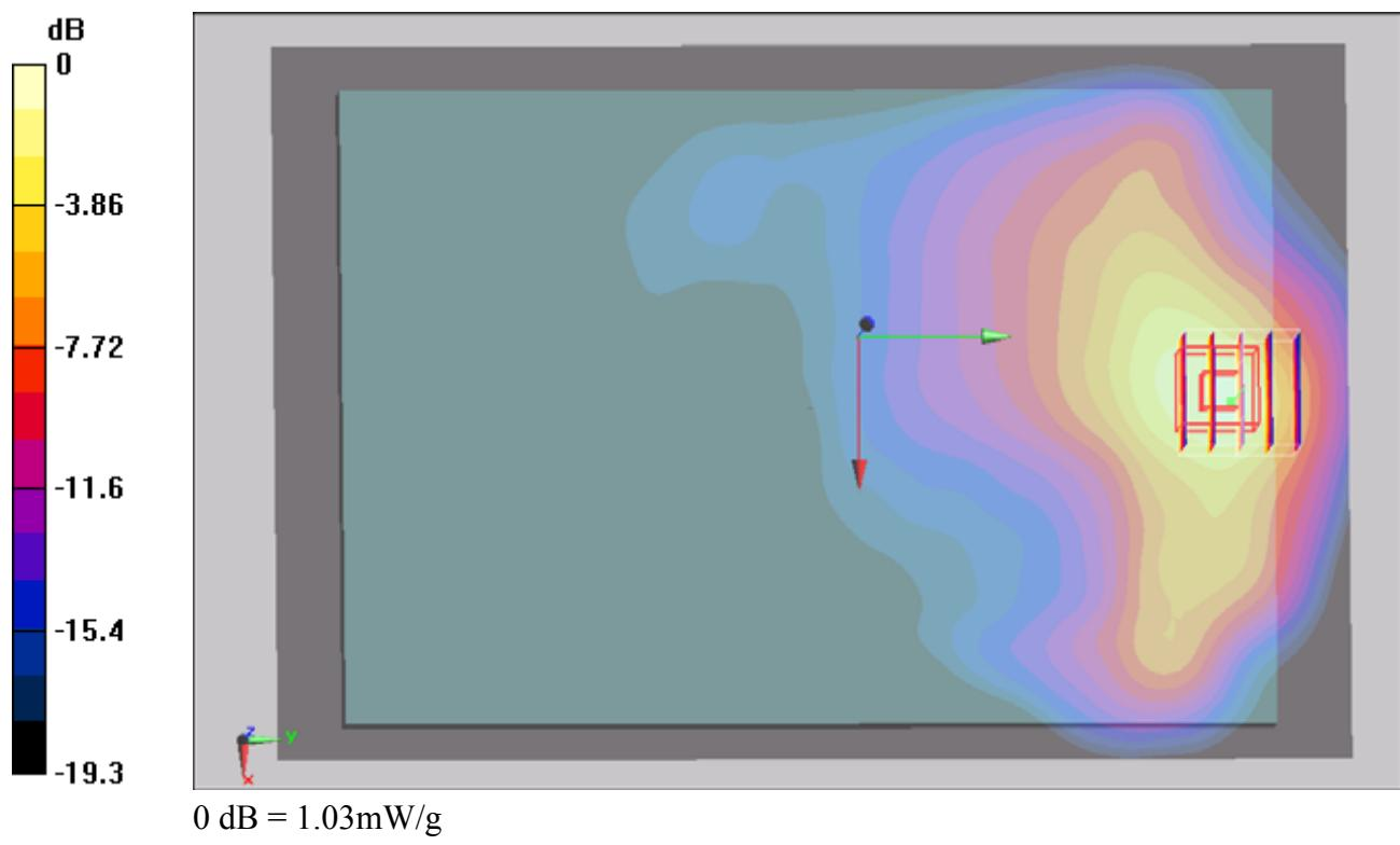
**#01 GSM1900\_GPRS10\_Bottom Face\_0.5cm\_Ch810\_Earphone\_2D****DUT: 132604-07**
