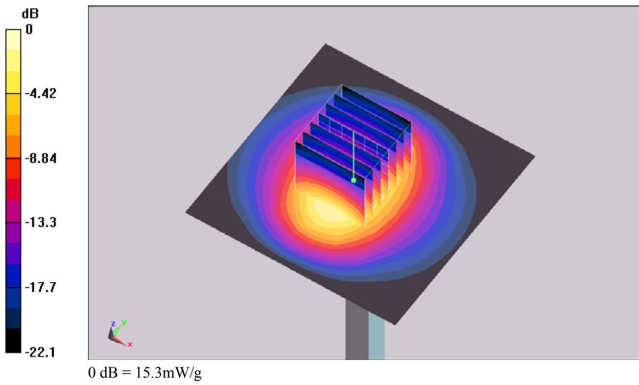
**System Check\_Body\_2450MHz\_110830****DUT: Dipole 2450 MHz**
