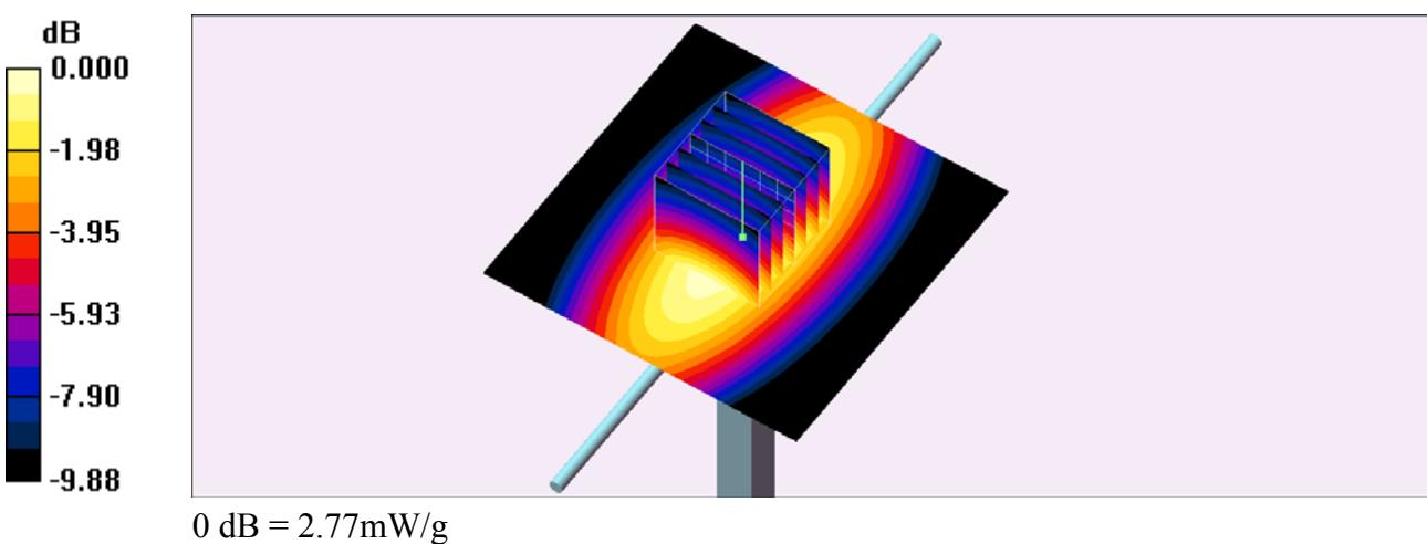
**System Check\_Body\_1900MHz\_110830****DUT: Dipole 1900 MHz**
