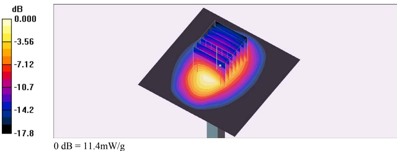
**System Check\_Body\_2450MHz\_110830****DUT: Dipole 2450 MHz**
