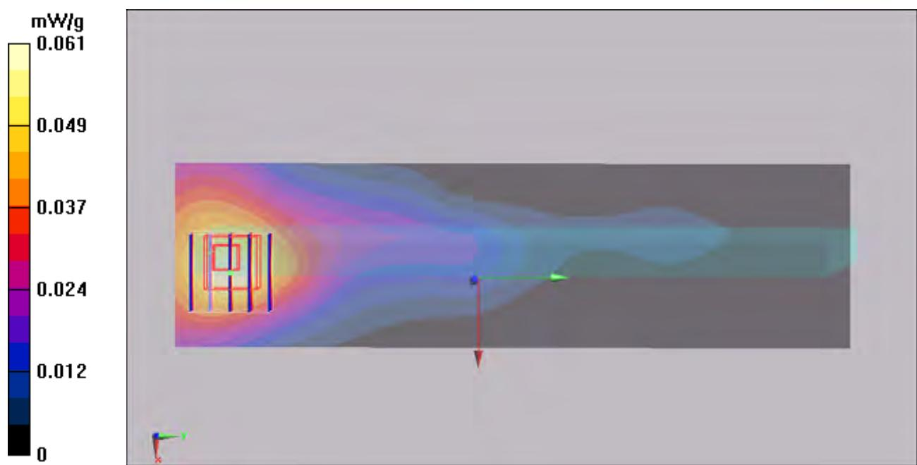
**#19 GSM850\_GPRS10\_Front Face\_10mm\_w/o Pw Reduction\_Ch251****DUT: 132604**
