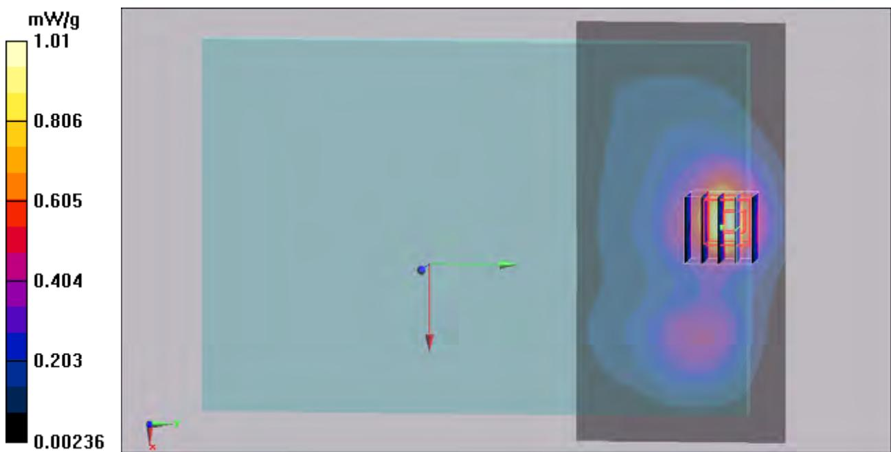
**#45 GSM1900\_GPRS10\_Rear Face\_0mm\_w/ Pw Reduction\_Ch810\_Earphone****DUT: 132604**
