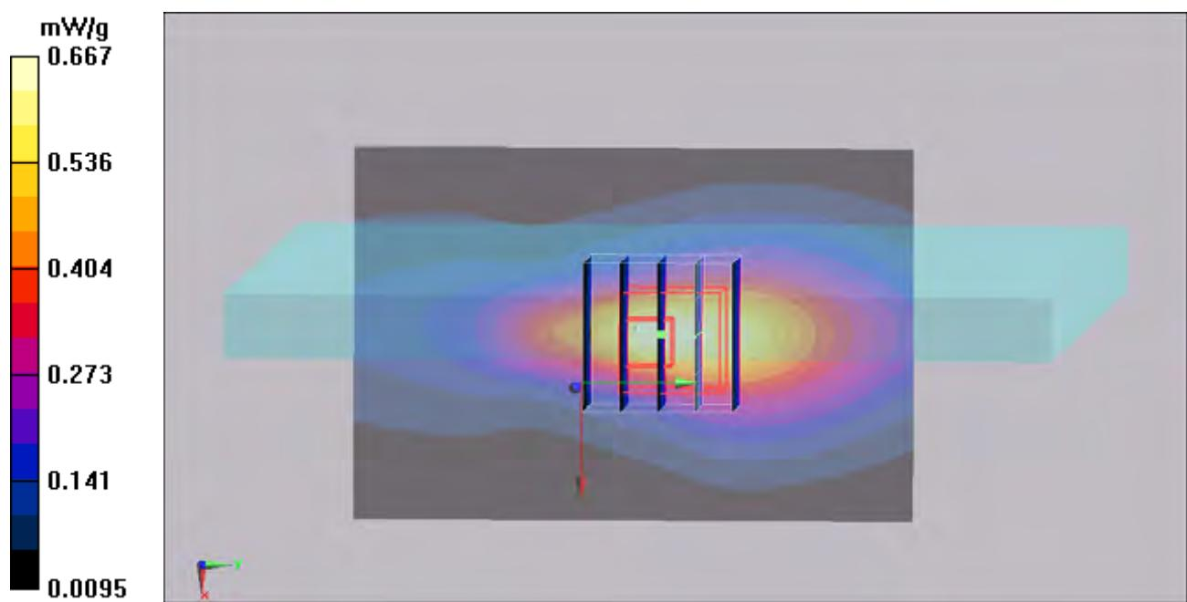
**#29 GSM850\_GPRS10\_Rear Face\_0mm\_w/ Pw Reduction\_Ch128\_Earphone****DUT: 132604**
