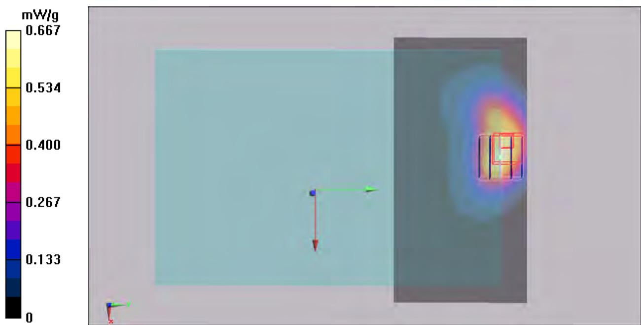
**#30 GSM850\_GPRS10\_Rear Face\_0mm\_w/ Pw Reduction\_Ch189\_Earphone****DUT: 132604**
