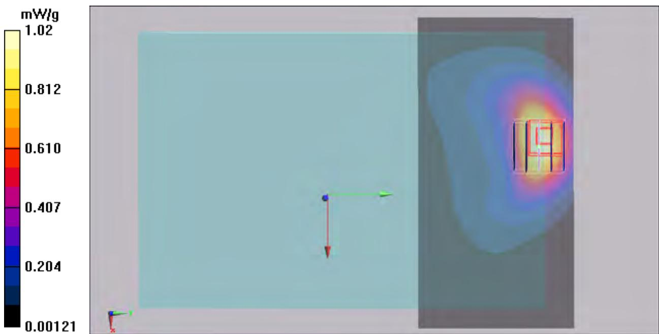
**#27 GSM850\_GPRS10\_Rear Face\_0mm\_w/ Pw Reduction\_Ch251\_Earphone****DUT: 132604**
