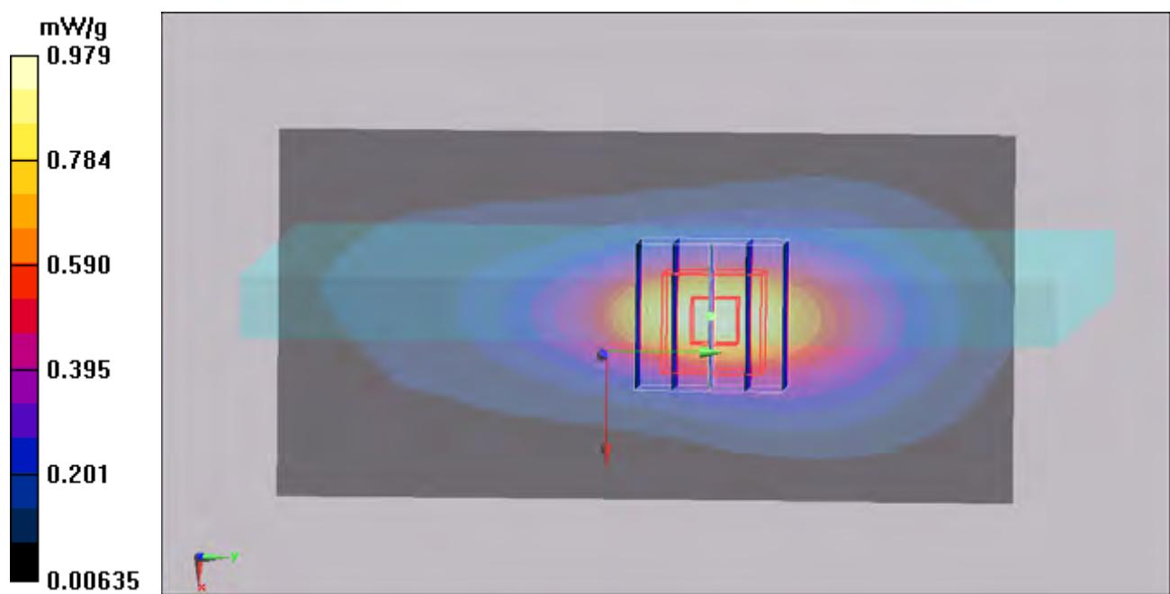
**#23 GSM850\_GPRS10\_Front Face\_10mm\_w/o Pw Reduction\_Ch128****DUT: 132604**
