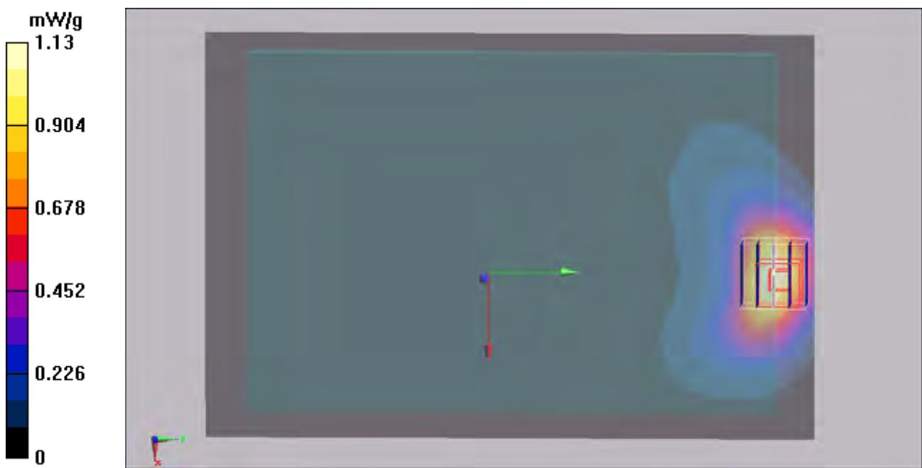
**#05 WCDMA V\_RMC12.2K\_Rear Face\_5mm\_w/o Pw Reduction\_Ch4182\_Earphone****DUT: 132604**
