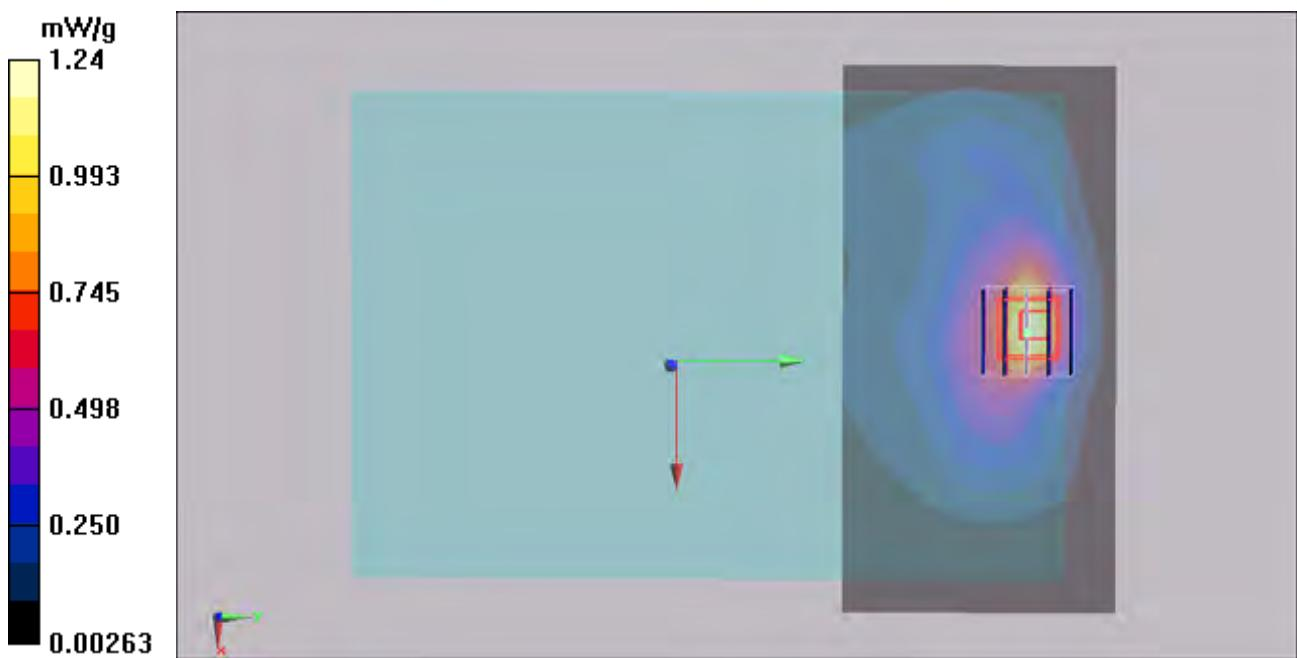
**#43 GSM1900\_GPRS10\_Rear Face\_5mm\_w/o Pw Reduction\_Ch512\_Earphone****DUT: 132604**
