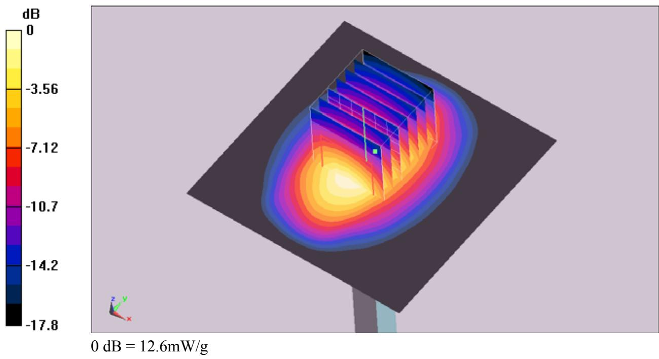
**System Check\_Body\_1900MHz\_110328****DUT: Dipole 1900 MHz**
