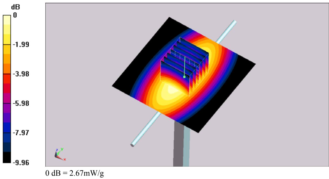
**System Check\_Body\_1900MHz\_110327****DUT: Dipole 1900 MHz**
