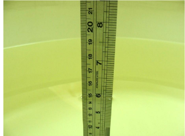
Fig 6.2 Photo of Liquid Height for Body SAR
