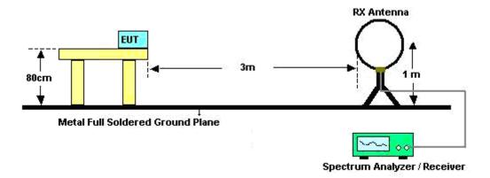
For radiated emissions from 30MHz to 1GHz
