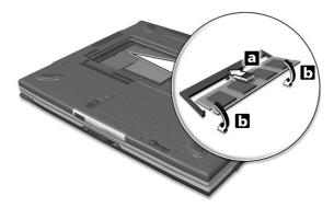
**4** Replace the memory cover and secure it with the screw.
