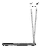
Doing otherwise will damage your keyboard when rotating the display screen.
