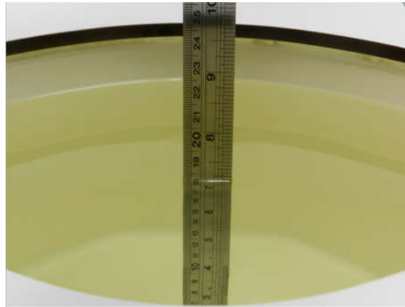
Fig 10.1 Photo of Liquid Height for Body SAR
