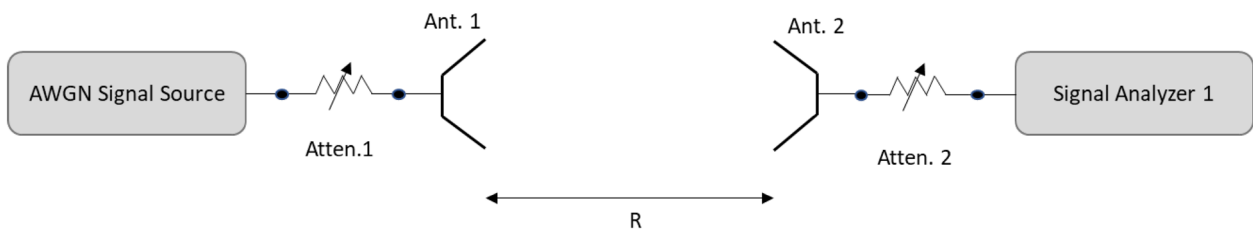
Figure 3. Contention-based protocol test setup, radiated method, power measurement
