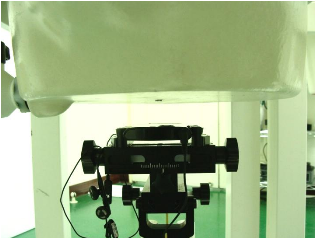
Bottom of the DUT with Phantom 1.5 cm Gap with Earphone 1 for Sample A
