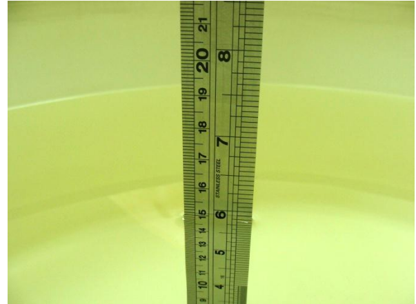
Fig 6.2 Photo of Liquid Height for Body SAR
