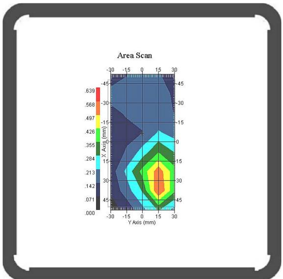
1 gram SAR value : 0.527 W/kg 10 gram SAR value : 0.325 W/kg Area Scan Peak SAR : 0.563 W/kg Zoom Scan Peak SAR : 0.865 W/kg
