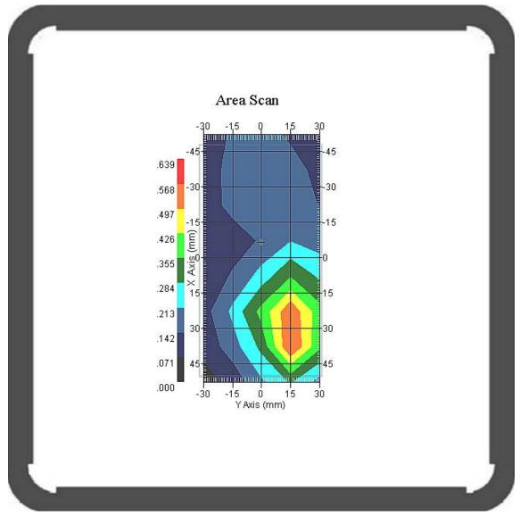
1 gram SAR value : 0.532 W/kg 10 gram SAR value : 0.327 W/kg Area Scan Peak SAR : 0.570 W/kg Zoom Scan Peak SAR : 0.863 W/kg
