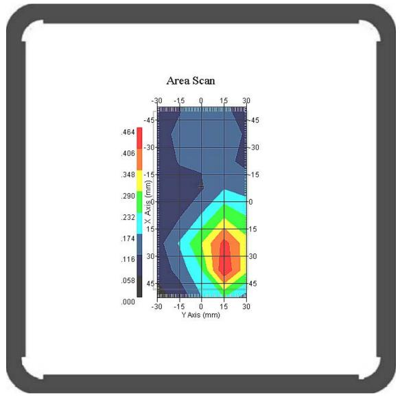
1 gram SAR value : 0.519 W/kg 10 gram SAR value : 0.312 W/kg Area Scan Peak SAR : 0.460 W/kg Zoom Scan Peak SAR : 0.842 W/kg
