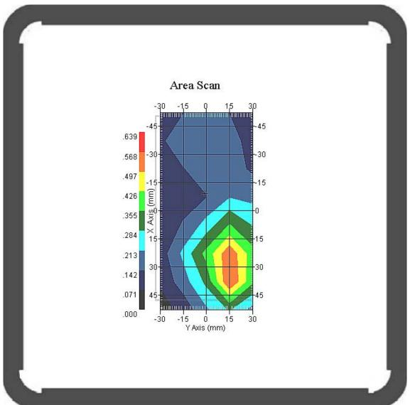
1 gram SAR value : 0.541 W/kg 10 gram SAR value : 0.325 W/kg Area Scan Peak SAR : 0.570 W/kg Zoom Scan Peak SAR : 0.877 W/kg
