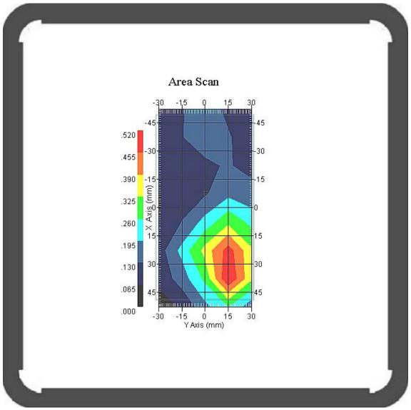
1 gram SAR value : 0.483 W/kg 10 gram SAR value : 0.275 W/kg Area Scan Peak SAR : 0.519 W/kg Zoom Scan Peak SAR : 0.820 W/kg
