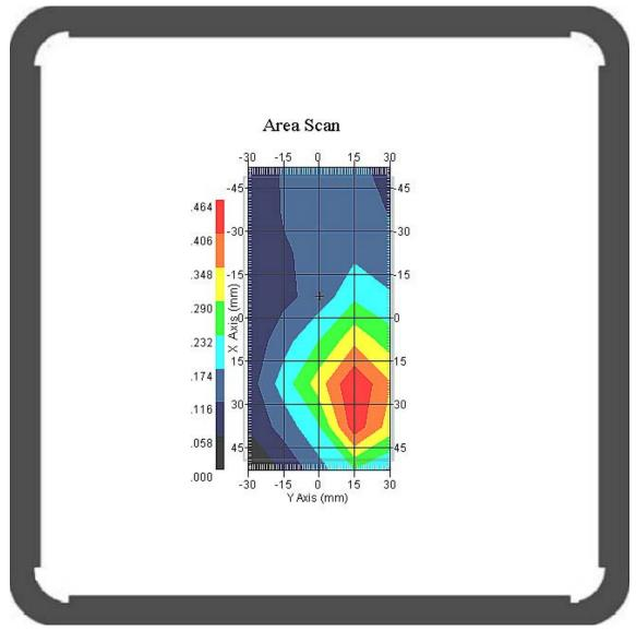
1 gram SAR value : 0.448 W/kg 10 gram SAR value : 0.226 W/kg Area Scan Peak SAR : 0.460 W/kg Zoom Scan Peak SAR : 0.769 W/kg
