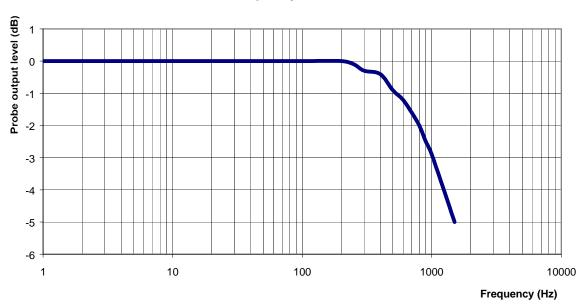
Video Bandwidth at 500 Hz1 dBVideo Bandwidth at 1000 Hz3 dB
