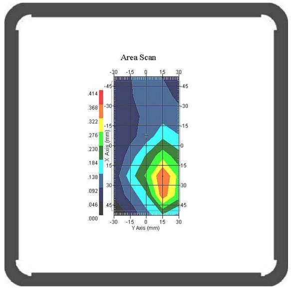
1 gram SAR value : 0.267 W/kg 10 gram SAR value : 0.175 W/kg Area Scan Peak SAR : 0.370 W/kg Zoom Scan Peak SAR : 0.640 W/kg
