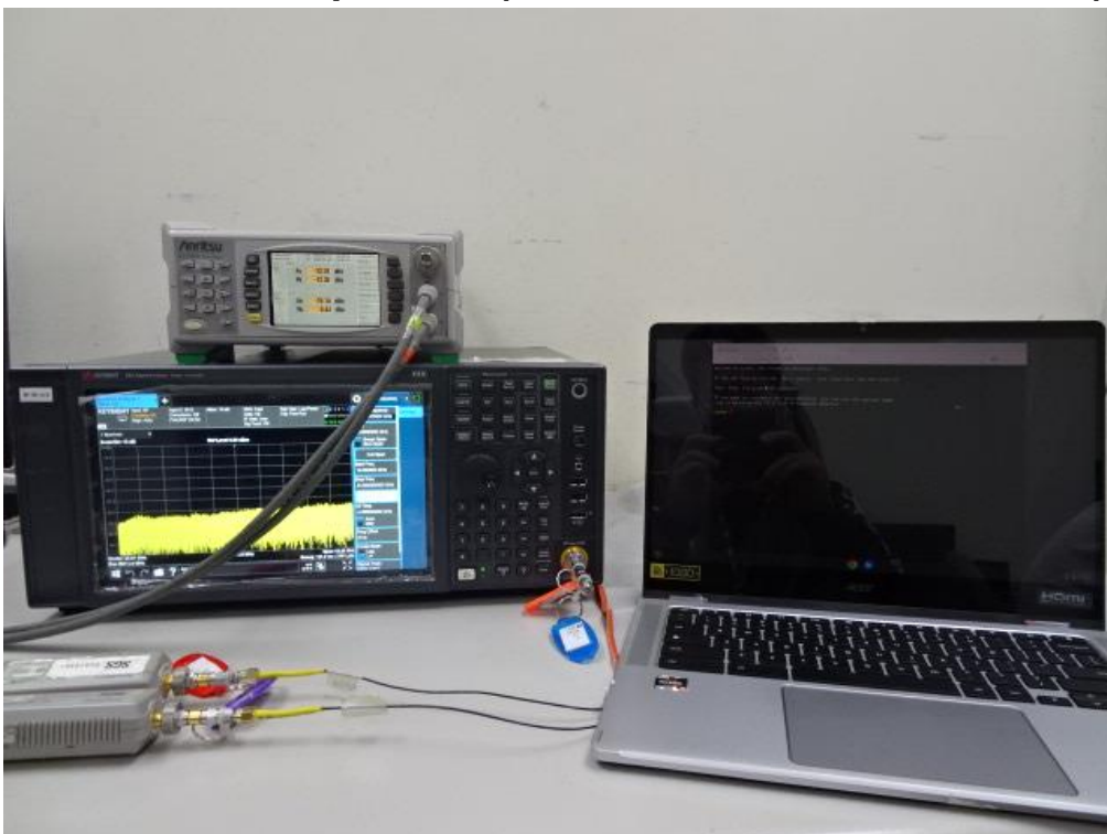
Conducted Setup Photo (Measurement at Antenna Port)
