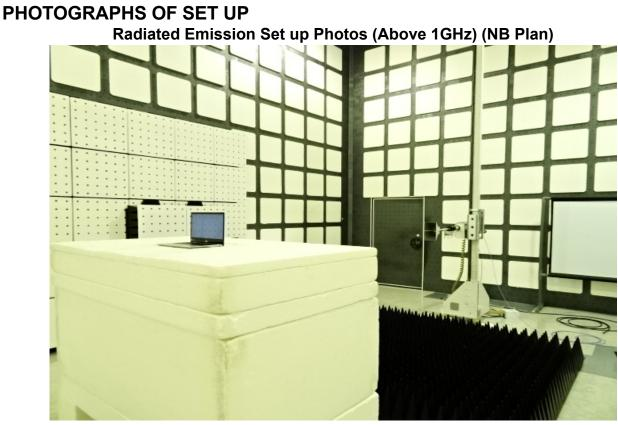
**Radiated Emission Set up Photos (Front View)**
