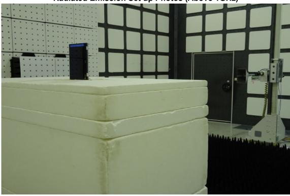
Radiated Emission Set up Photos (Front View)
