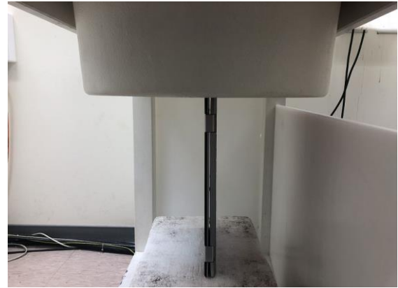
Fig.6 EUT Right side to flat phantom
