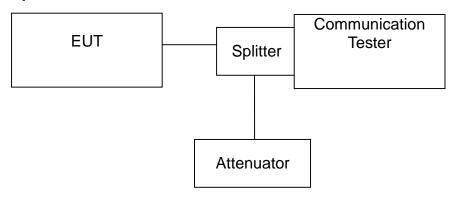
Note: Measurement setup for testing on Antenna connector
