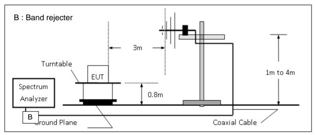
Radiated Emission Test Set-UP Frequency Over 1 GHz
