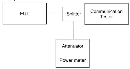
**Note:** Measurement setup for testing on Antenna connector
