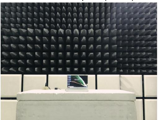
Radiated Emission Set up Photos (Front View)
