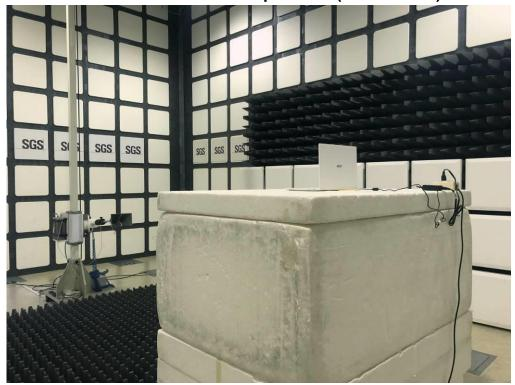
Radiated Emission Set up Photos (Front View)
