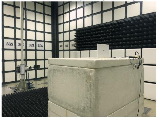
Radiated Emission Set up Photos (Front View)
