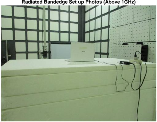
Radiated Bandedge Set up Photos (Above 1GHz)
