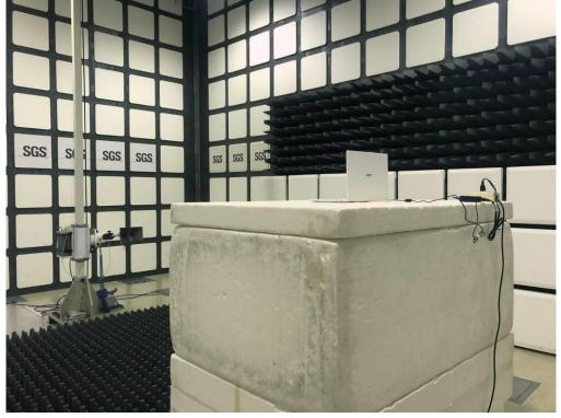
Radiated Emission Set up Photos (Front View)
