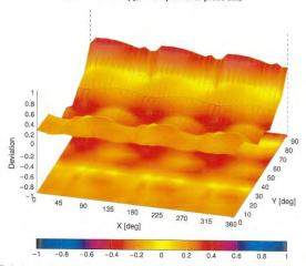
Probe isotropy for  $E_{tot}$ : probe rotated  $\phi = 0^{\circ}$  to 360°, tilted from field propagation direction  $\vec{k}$ Parallel to the field propagation ( $\psi$ =0° - 90°) at 30 GHz: deviation within ±0.45 dB Parallel to the field propagation ( $\psi$ =0° - 90°) at 60 GHz: deviation within ±0.44 dB
