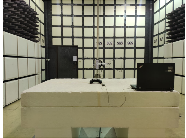
FCC 15_247 BLE Radiated_Setup
