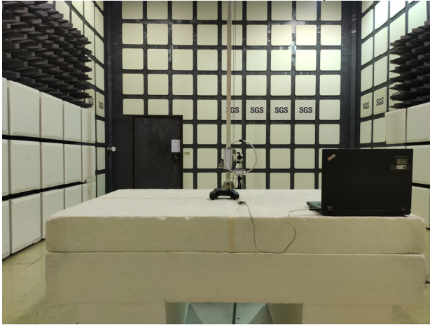
FCC 15_247 BLE Radiated_Setup
