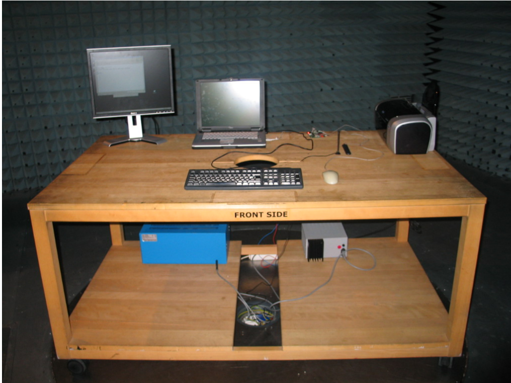
Photo 2: Test setup for radiated measurements
