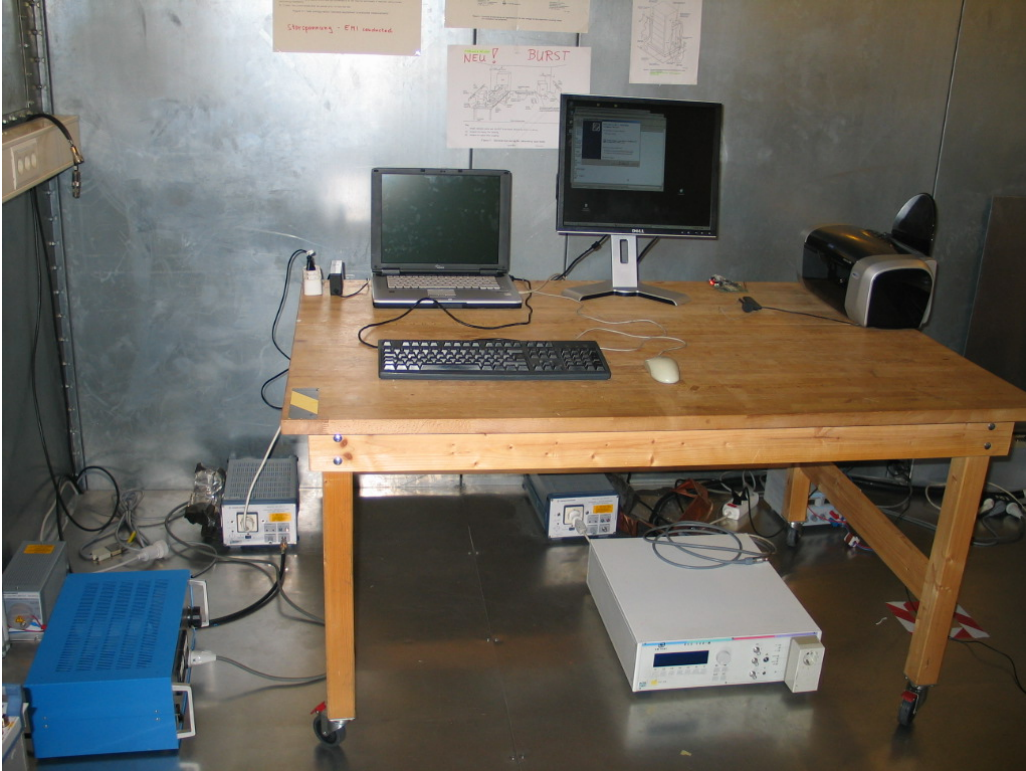
Photo 1: Test setup for conducted measurements
