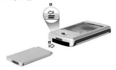
**NOTE:** To take the battery pack out, first slide the battery release switch to the unlocked position, then pull the battery pack out of the bay.
