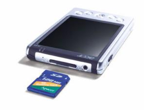
3 Push the card into the slot using your finger until you feel the card lock and hear an audible system sound. This indicates that the card is properly seated within the slot.
