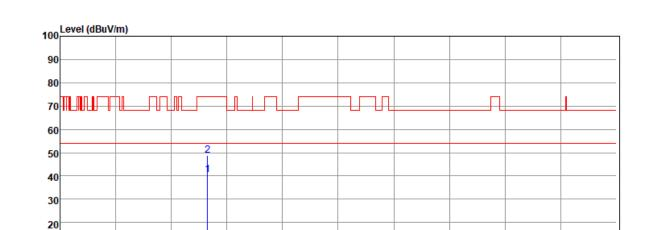
0 1000 8800. 32200. 40000 Frequency (MHz) Freq. Detector Spectrum Factor Actual Limit Margin Mode Reading Level FS @3m PK/QP/AV dΒ MHz dBµV dB dBµV/m dBµV/m 11340.00 27.84 12.50 40.34 54.00 -13.66 Average 11340.00 Peak 36.38 12.50 48.88 74.00 -25.12
