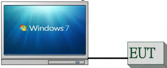
Fig. 2-2 Conducted (Antenna Port) Emission Configuration
