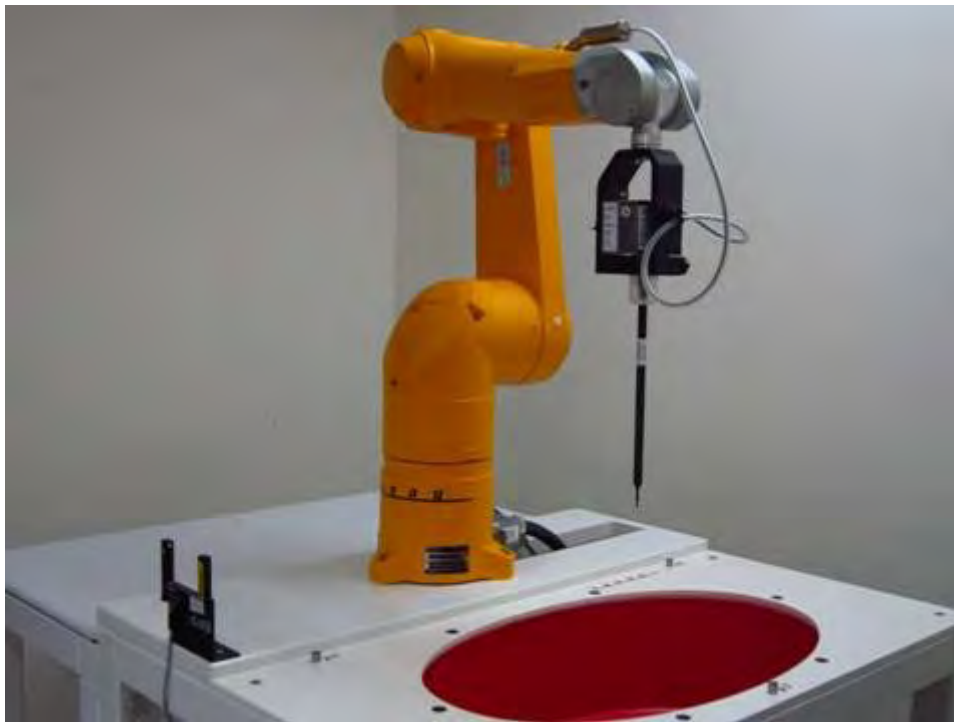
Fig.1 Photograph of the SAR measurement system
